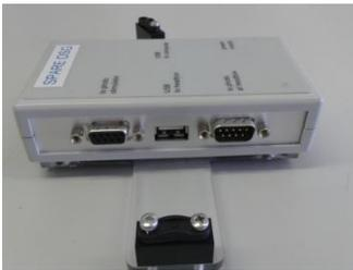
Interface between computer and headbox. Power supply connected to USB power adapter.
